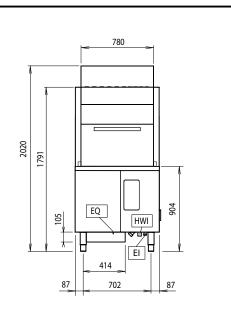
Drain Electrical inlet (power) FΩ **Electrical Outlet** HWI Hot water inlet Detergent connection Rinse aid connection
